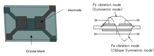
Fig.2: MCF configuration and Vibration mode outline
