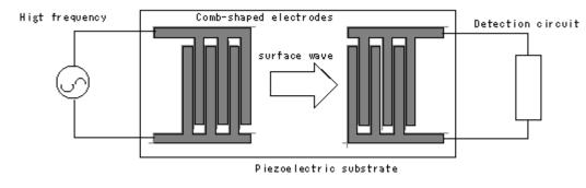
Fig.1: SAW Filter configuration
